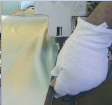
Welding the rim-reinforcement with the vinyl
