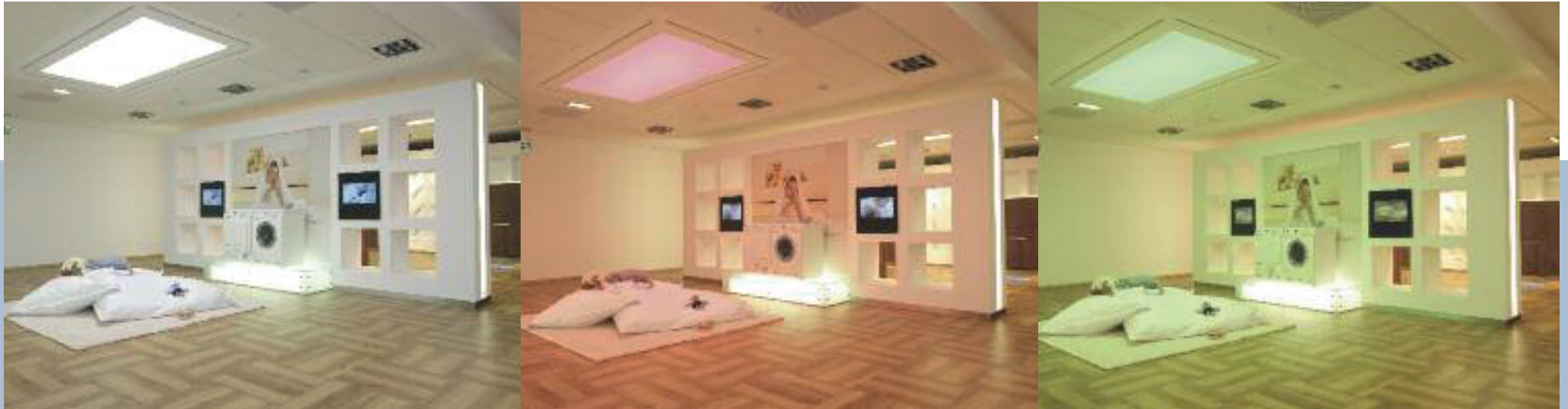
Miele showroom , headquarter Gütersloh – ca. 20 RGB-lighted ceilings create a light atmosphere in every color desired. Adjustable rim construction with a pull-out rope and RGB-T5 light control via a BUS system
